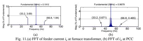
Fig. 11(a), (b), show two frequencies 33.2 Hz and 6 6.8 Hz because 16.8 Hz signal was impregnated during resistance modulation. For this reason, the furnace feeder is considered as the source of super and SSFs and the EAF can be considered as the source current which disturbs the electromagnetic torque in the synchronous generator.
