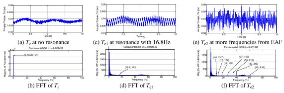
Fig. 14. Electromagnetic torque with EAF in the system
