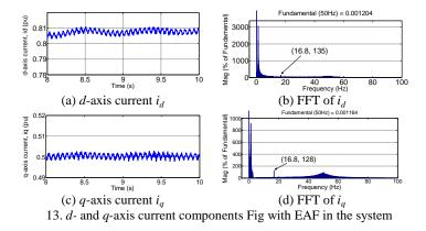
Fig. 13 explains the dq-axis current component s with EAF in the system. Since the frequency of the modulating signal is 16.8 Hz, it is seen in Fig. 13(b), (d) which also prove of having 16.8 Hz frequency component as dominant. Comparing dq-axis current components in Fig. 12(a), (c) with dq-axis currents in Fig. 13(a), (c), it is deducible that amplitude of oscillation of dq-axis currents are larger with EAF.
