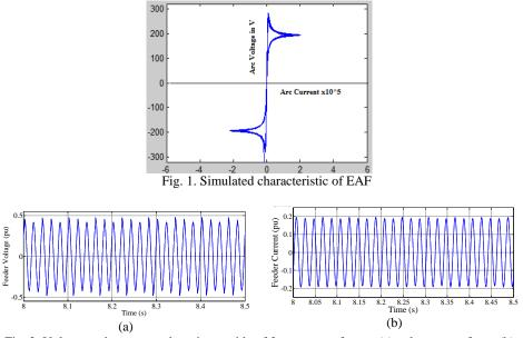
Fig. 2. Voltage and current at the primary side of furnace transformer (a) voltage waveform, (b) current waveform
