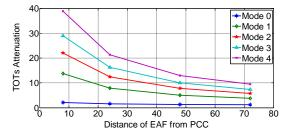
Fig. 17. Torque ratio (resonant to non-resonant condition) due to different distances between PCC and EAF
